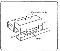
To Attach the Extension Table (for flat-bed sewing)
